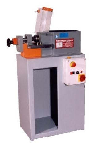
This machine has been realised for cutting stripes of different measures without the necessity of changing the fixed equipment of blades.
